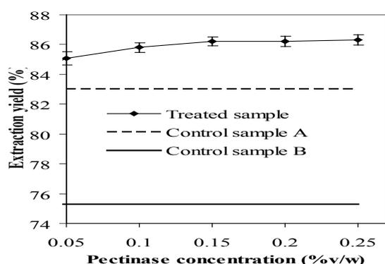
**Figure 1.** Effect of enzyme concentration on extraction yield of the simultaneous treatment of acerola mash by ultrasound and pectinase preparation
