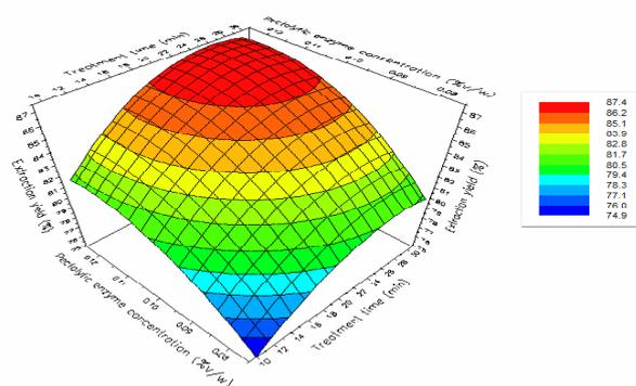
**Figure 3.** Response surface plot for extraction yield in the simultaneous treatment of acerola mash by ultrasound and pectinase preparation
