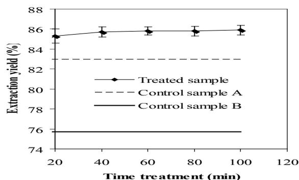
**Figure 2.** Effect of pectolytic time on extraction yield of the simultaneous treatment of acerola mash by ultrasound and pectinase preparation
